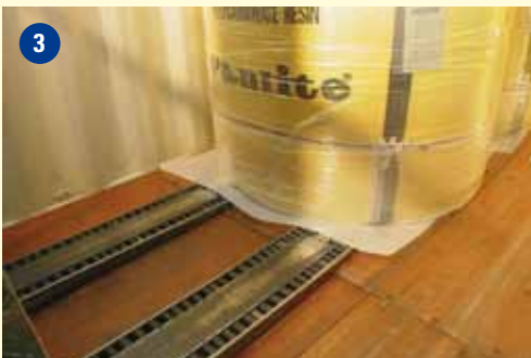
3 Lifting up goods directly from the floor
